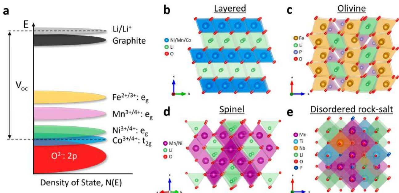
**Figure 2.** (a) Redox energies of cobalt (Co), nickel (Ni), manganese (Mn), and iron (Fe) relative to those of lithium (Li) and graphite. Crystal structures of (b) layered oxide  $\text{LiNi}_x\text{Mn}_y\text{Co}_z\text{O}_2$ , (c) olivine  $\text{LiFePO}_4$ , (d) spinel  $\text{LiNi}_x\text{Mn}_y\text{O}_4$ , and (e) disordered rock-salt  $\text{Li}_2\text{Mn}_w\text{Nb}_x\text{Ti}_y\text{O}_{3-z}\text{F}_z$ .
